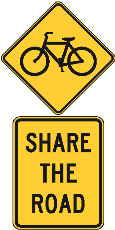
Figure 10. 'Share the Road' signage can be used along roadways to indicate preferred cycling routes.
