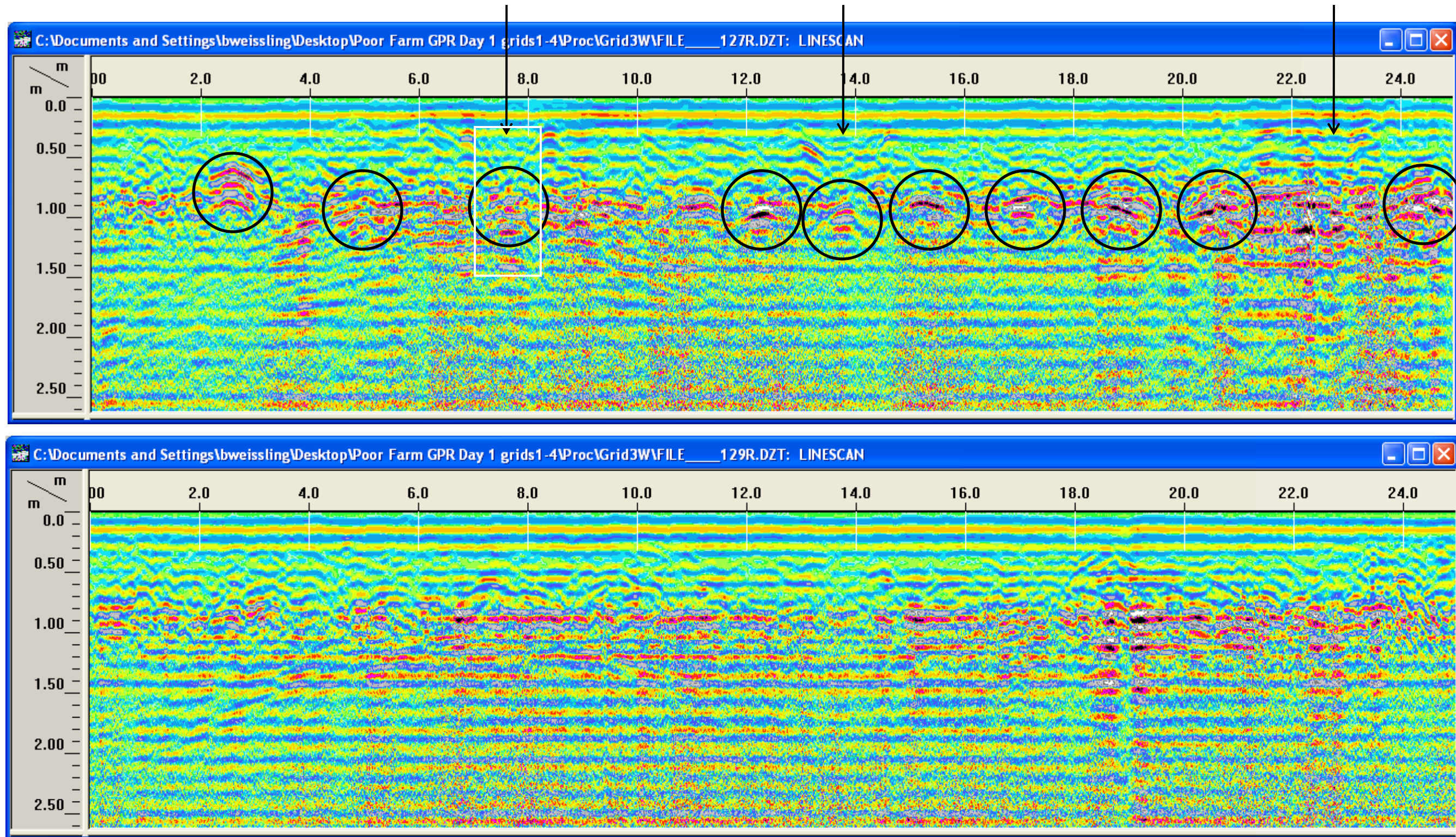
Figure 26. Radar profile line 127 (top) of grid 3 showing anomalies consistent in both depth and spacing with burials.
