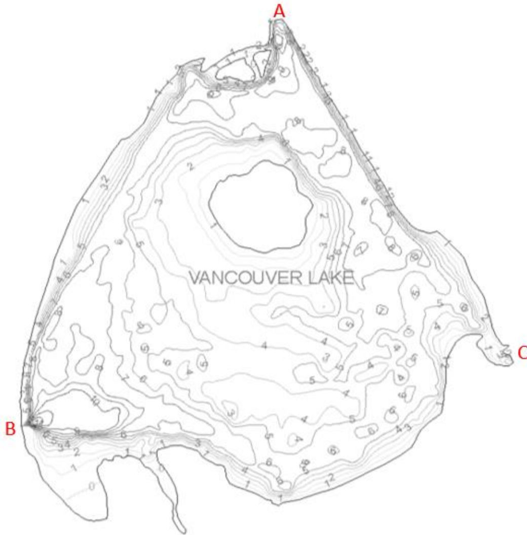
Figure 4. Vancouver Lake’s relative water depth contours in feet based on GPS and depthfinder data collected by Spenser Vines as part of his Eagle Scout project work (October 11, 2004). Water flows into the lake from Burnt Bridge Creek (Point C), and sometimes from Lake River (Point A), and the flushing channel (Point B). Water only flows out via Lake River (Point A).
