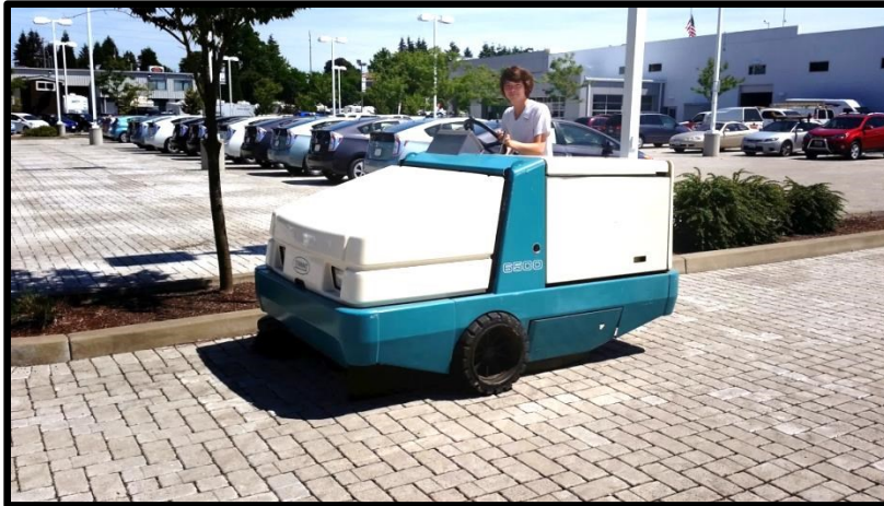
Figure 7 Paver cleaning with a Tennant 6500 vacuum filtering sweeper
