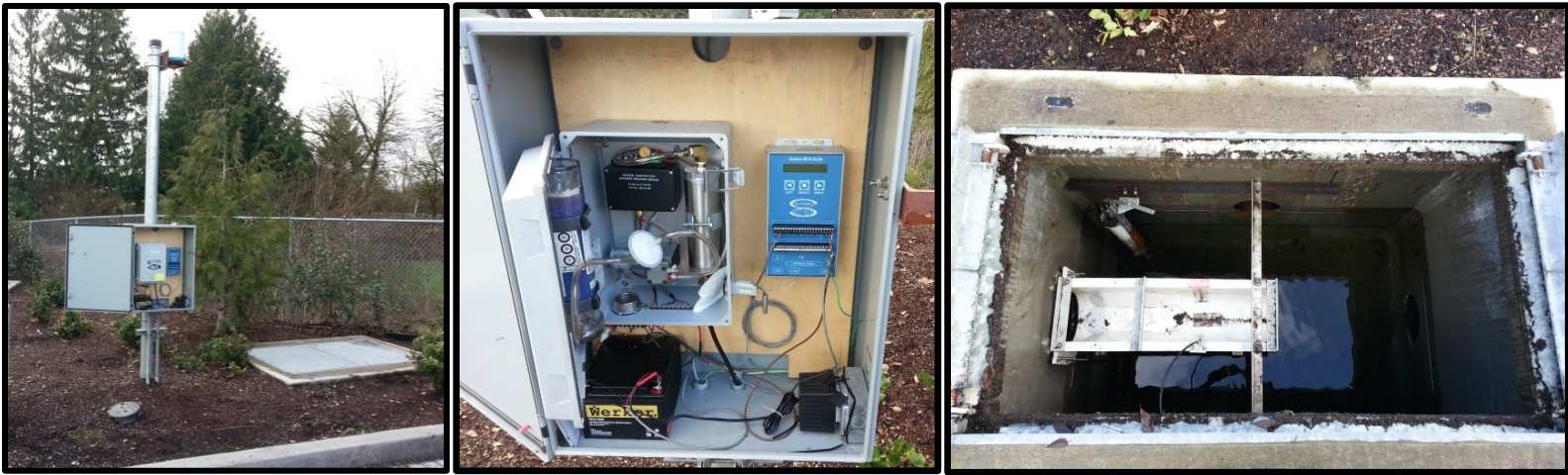
Figure 8. Continuous monitoring data collection platform: left - overall system with electronics enclosure, rain gage and closed vault; center – close-up of electronics enclosure with bubbler and data logger, and right –opened vault showing flume and crest gage
