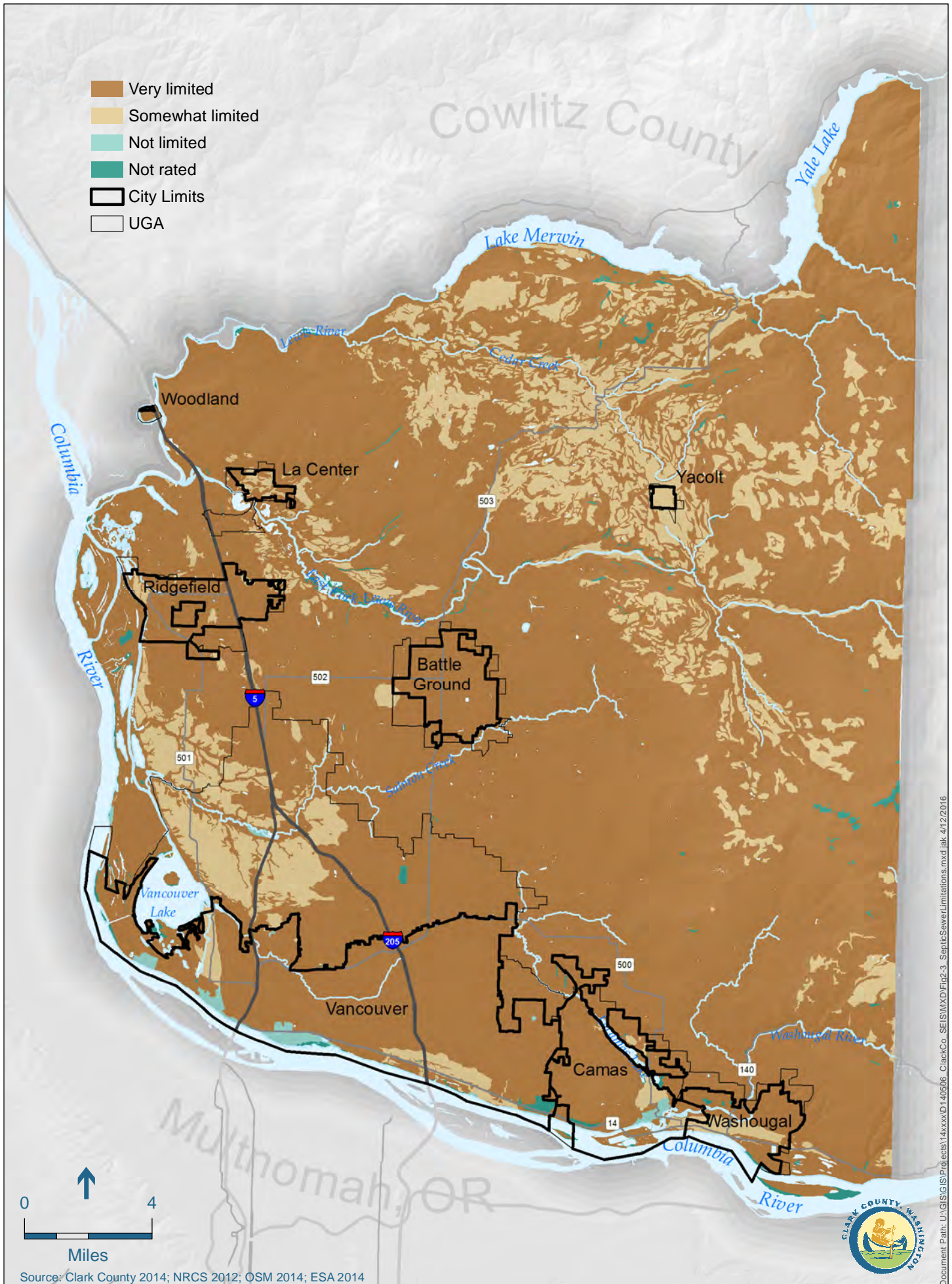
Figure 2-3: Soil Limitations to Septic Sewer Systems
