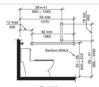
Fig. 604.5.1 Side Wall Grab Bar for Water Closet
