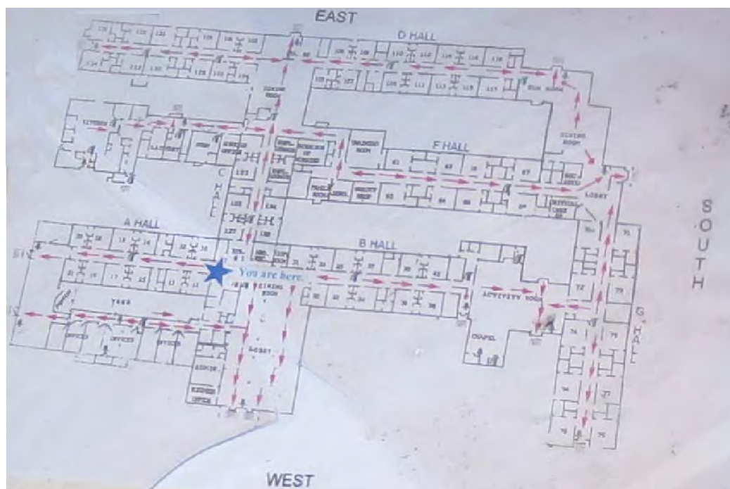
Figure 34. Emergency Exit Floor Plan for the West Rest Haven (Source: CSB)
