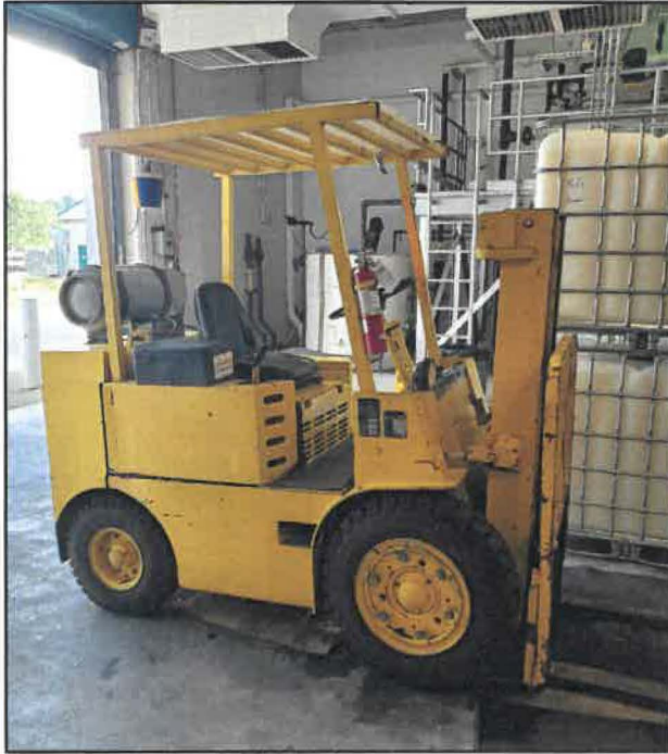
Old forklift with 4,000-pound lift capacity
