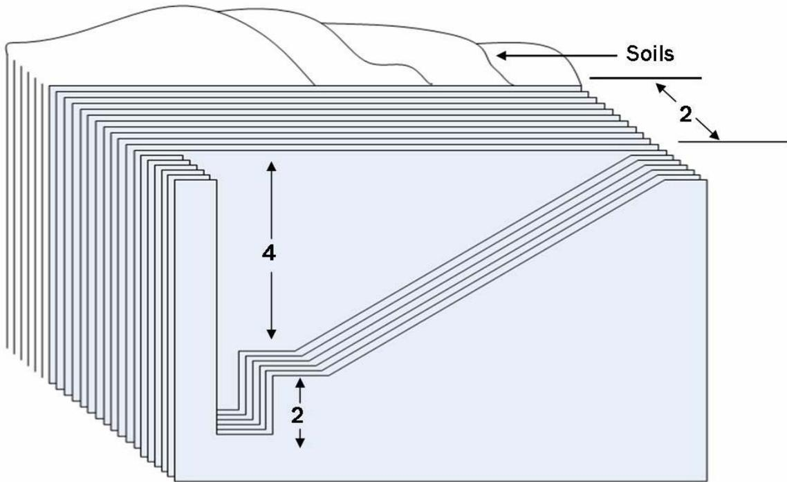
1. For a conventional system on a flat site without a cap, the profile hole depth of 5 feet would be required, if a restrictive layer was not encountered.
