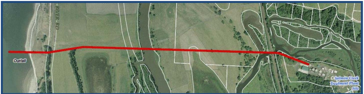
*Existing Salmon Creek Treatment Plant Effluent Pipeline/ Outfall in Columbia River*
