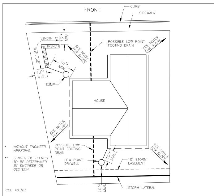
ALL LOTS WITHIN THE URBAN GROWTH AREA MUST BE DESIGNED TO PROVIDE POSITIVE DRAINAGE FROM BOTTOM OF FOOTINGS TO AN APPROVED STORMWATER SYSTEM. POSITIVE DRAINAGE MAY BE ACCOMPLISHED BY SWALES, DRYWELLS, FRENCH DRAINS, LATERALS TO THE STREET, LATERALS BEHIND THE CURB OR WITHIN A PUBLIC UTILITY EASEMENT, AN APPROVED SYSTEM, IN THE SIDE OR REAR SETBACK, OR SOME OTHER METHOD ACCEPTABLE TO THE RESPONSIBLE OFFICIAL.
