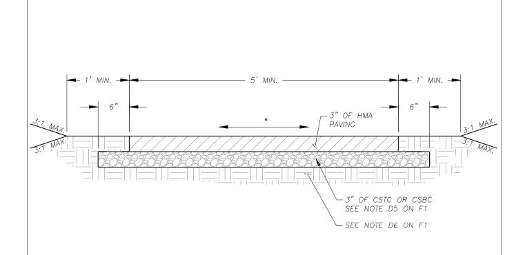
\* 1.5% OR FLATTER RECOMMENDED FOR DESIGN/FORMWORK (2% MAX)
