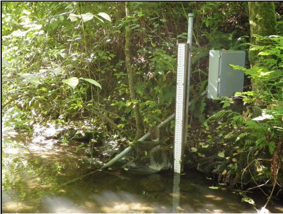
Figure 2 Cougar Creek hydrology monitoring station (CGR018) staff gage, diagonal pipe housing pressure transducer, and secure equipment shelter
