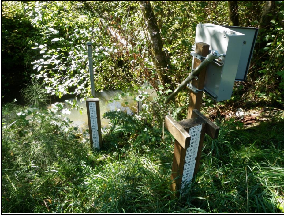
Figure 1 Whipple Creek hydrology monitoring station (WPL048) staff gages, transducer pipe, and accessible equipment shelter
