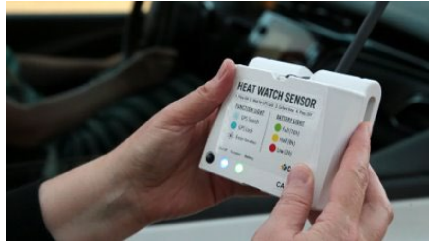
Pictured above: Heat Watch temperature sensor
